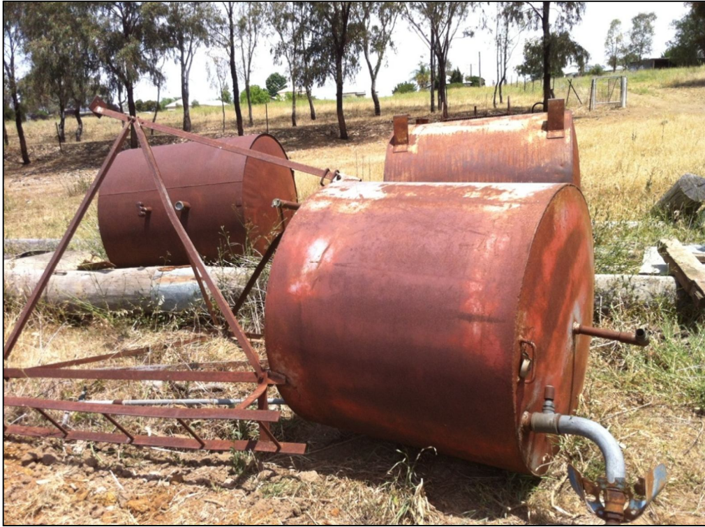
Plate 5 – Rusted approximately 1000L empty tanks observed at Location 10.
