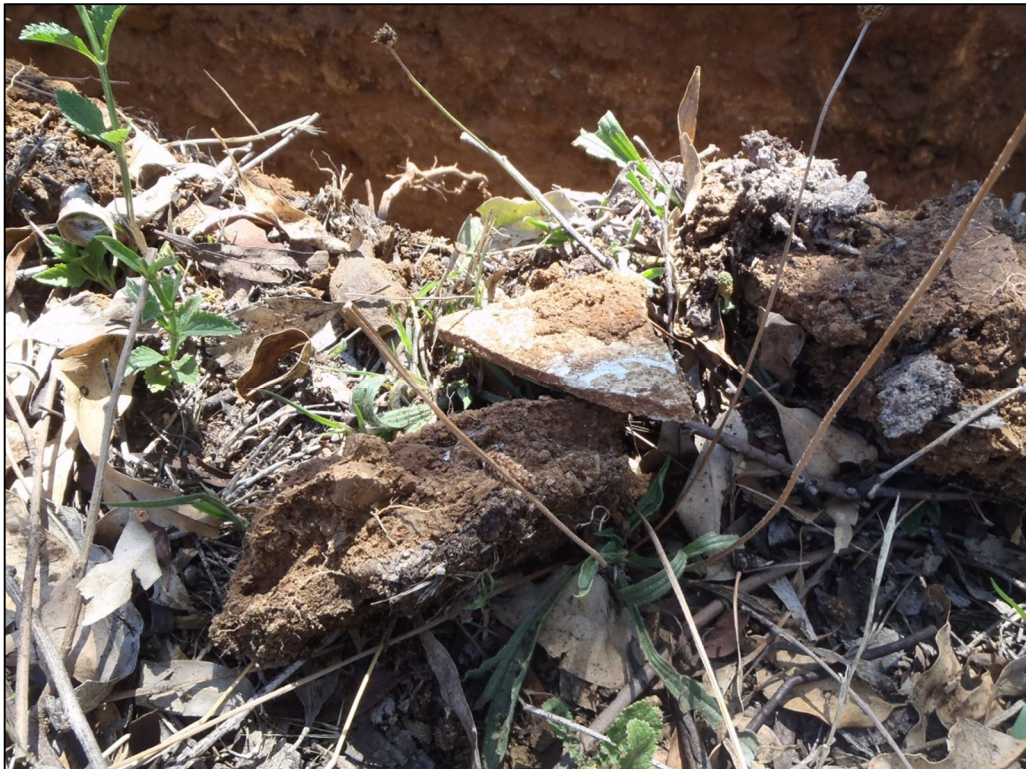
Plate 16 – ACM fragment observed in the top 0.1m of testpit TP5.
